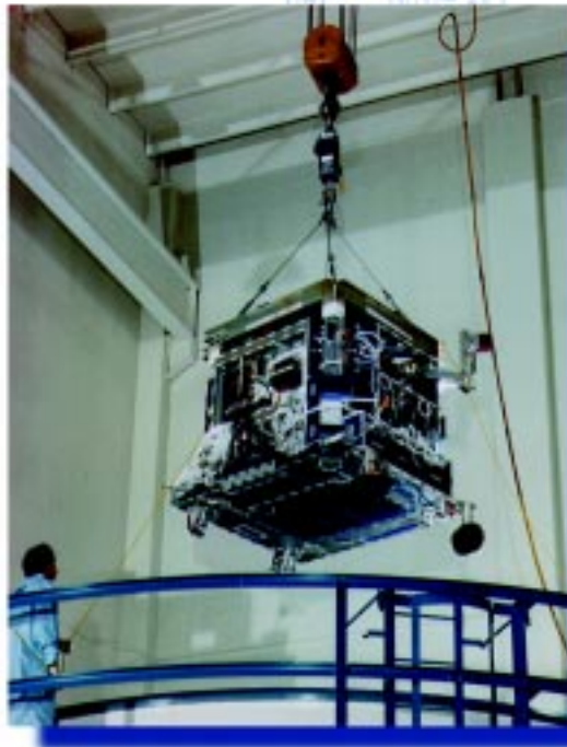
The Radarsat spacecraft bus is lowered into a thermal vacuum chamber in Ball's test facilities in Boulder, Colorado.
