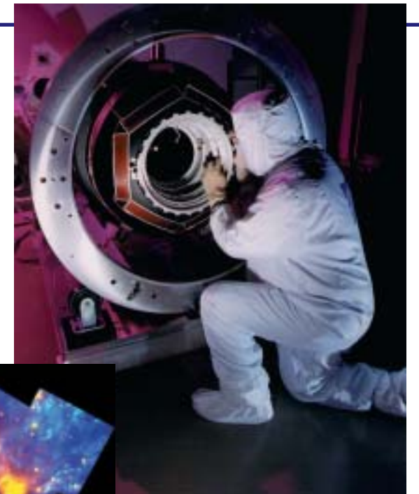
The filter wheel housing of the NICMOS dewar allows scientists to choose different filters for each image.
