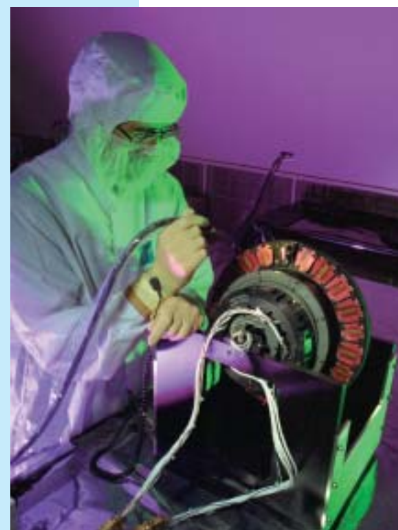
The STIS optics ring is made up of a selection of mirrored optics, allowing different views of space.
