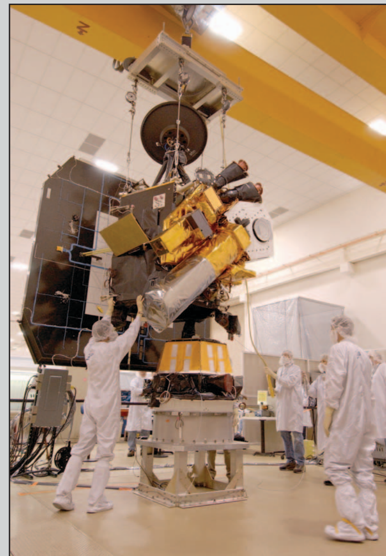
A "stack" procedure in Ball Aerospace's cleanroom matched both spacecraft into their launch configuration.
