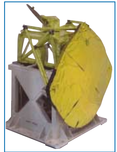
The AMSR-E instrument with its antenna in its stowed configuration for the Aqua launch. (Photo courtesy of NASDA.)
