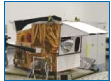
The MODIS instrument with the radiative cooler door open. (Photo courtesy of Raytheon.)
