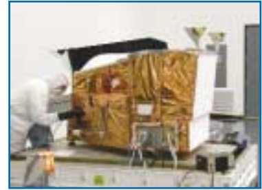
The MODIS instrument with the radiative cooler door closed. (Photo courtesy of Raytheon.)
