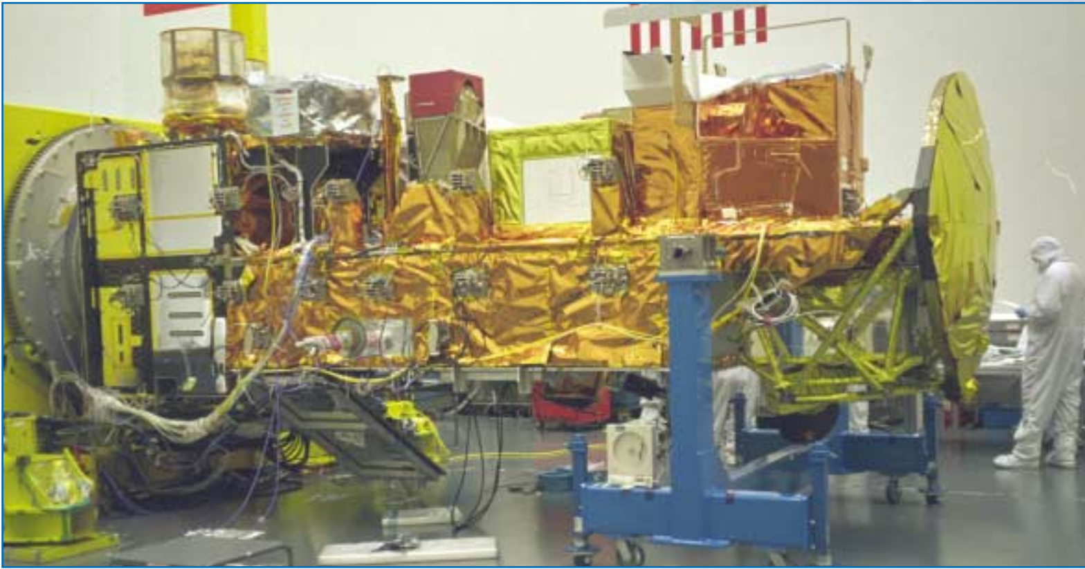
Solar array side prior to the installation of the solar array panel. (Photo by Claire Parkinson.)
