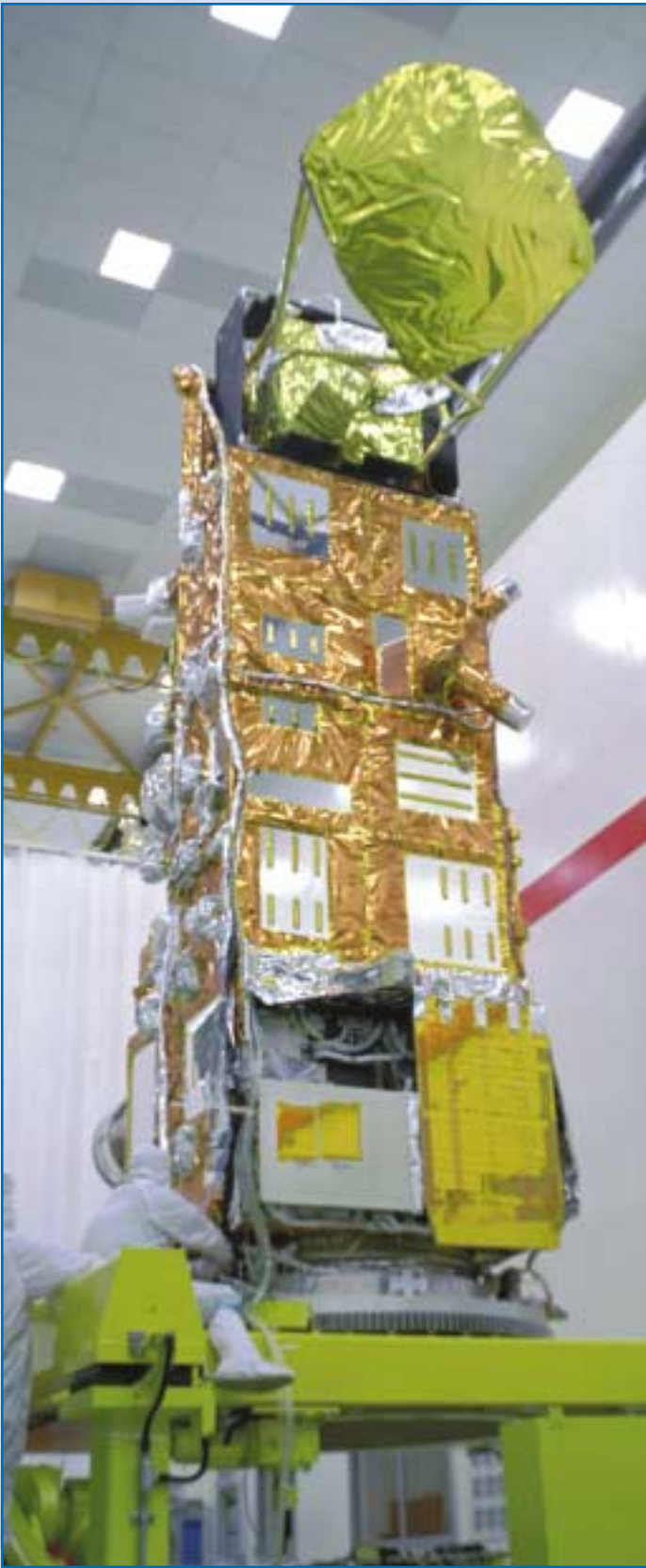
Space-viewing side, with the star trackers prominent in the middle right and the AMSR-E antenna prominent at the top. (Photo by Sally Ariestei.)
