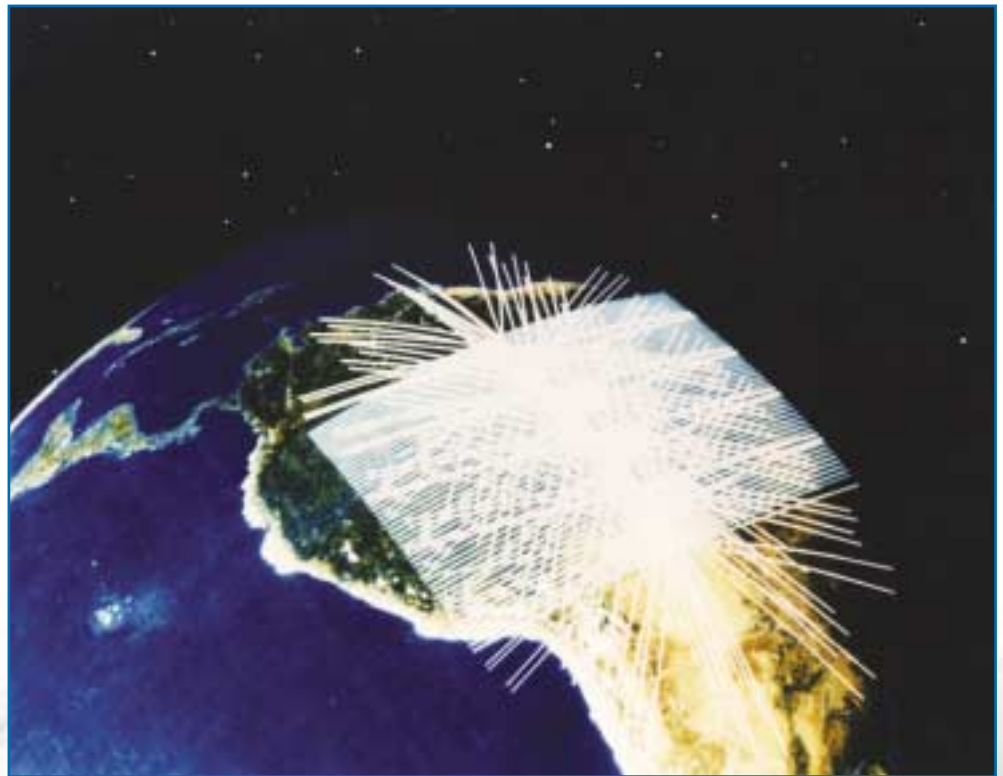
Schematic of the CERES scan lines as the Aqua satellite passes over South America. The scan lines from the CERES operating in the fixed azimuth plane scanning mode are all perpendicular to the orbital ground track, systematically lined up like a TV raster scan. The scan lines from the CERES operating in the rotating azimuth plane scanning mode appear closer to pinwheels when mapped onto the Earth, sampling a wide range of viewing angles. (Schematic courtesy of TRW.)
