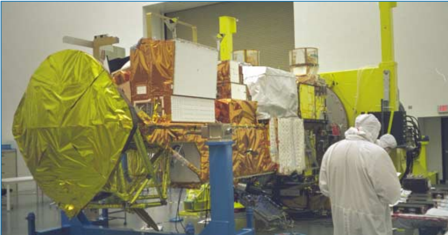
Side opposite the solar array, with, left to right, the AMSR-E, MODIS, AMSU-A1, AIRS (with a white protective covering), and CERES (with purge covers) instruments partially visible. (Photo by Claire Parkinson.)
