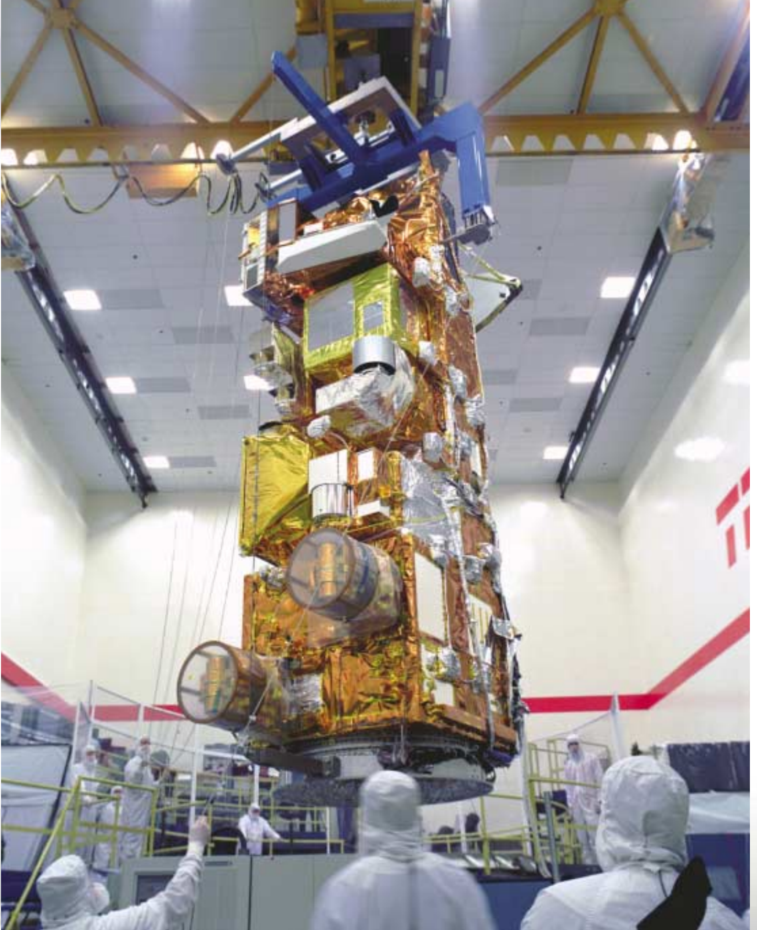
Aqua at TRW, August 2001, being positioned for lowering into the thermal vacuum chamber. (Photo by Sally Aristei.)
