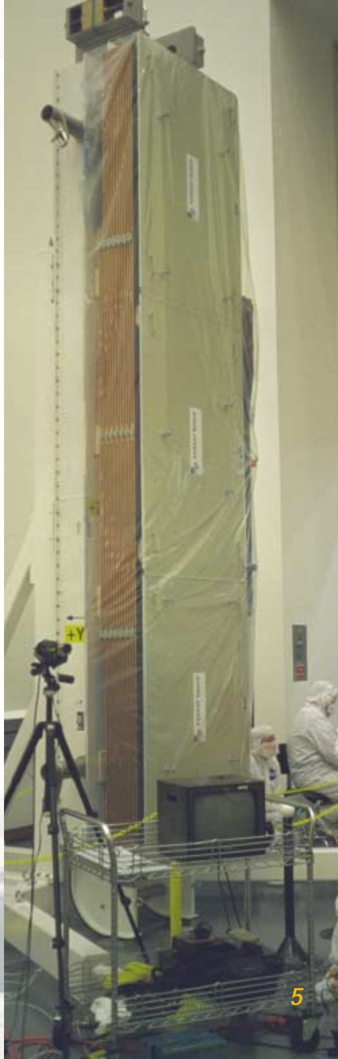
Aqua's solar array prior to its final installation on the Aqua spacecraft. After launch, the array will be unfurled, stretching 14 m outward from the spacecraft bus. (Photo by Claire Parkinson.)
